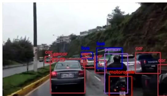
Figure 28: Tracking of vehicle movement using Artificial Intelligence.
