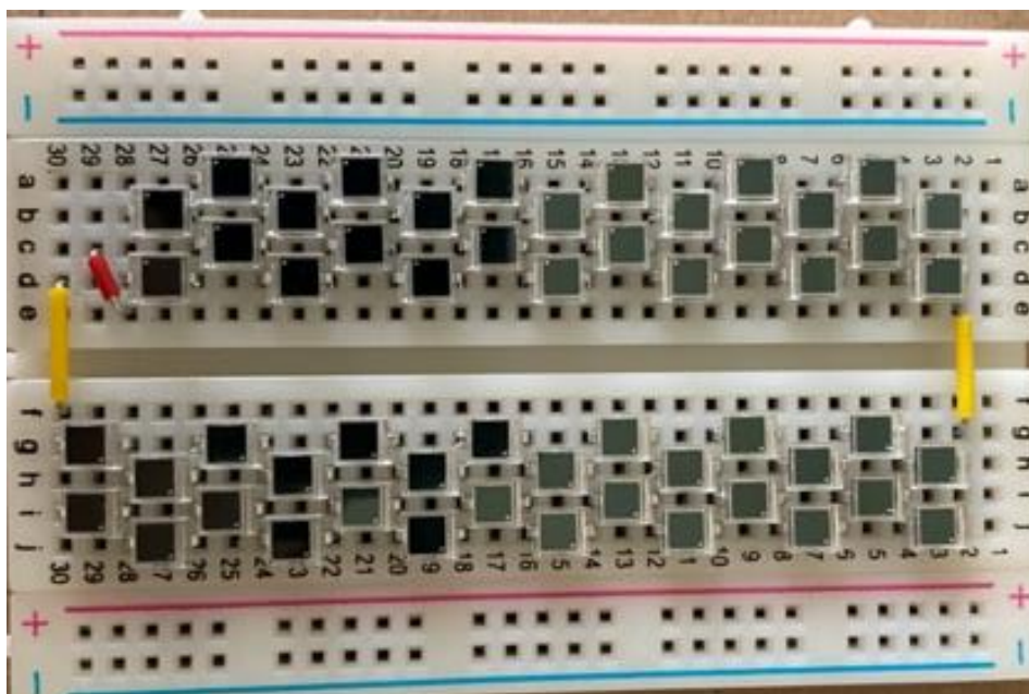
Image 3: Arrangement of photodiodes on a breadboard
