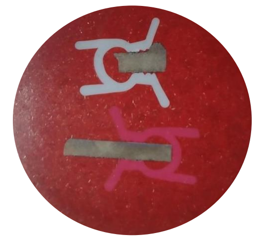
Embedded samples used for material analysis
