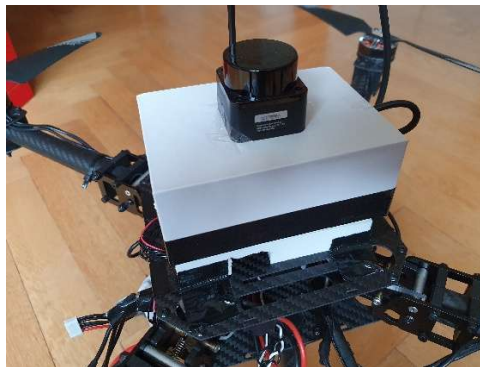
Picture 3: Polystyrene tower housing Raspberry Pi and Pixhawk
