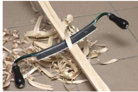
Abb.21: Ziehmesser, Eugster, Simon A.: Drawknife, working on a hazelnut flat-bow, 20.08.2009, Online: < https://commons.wikimedia.org/wiki/File:Working_with_Drawknife.jpeg >, Stand: 29.12.2019.
